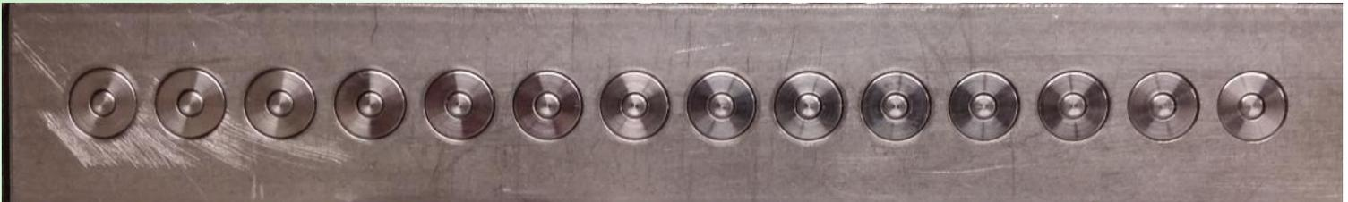
A200 VALVE BLOCK AFTER 24 MONTHS IN FIELD (WATER-BASED INK)
