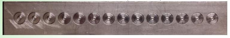
A200 VALVE BLOCK AFTER 24 MONTHS IN FIELD (WATER-BASED INK)
