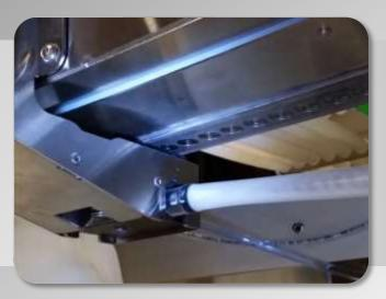
At the heart of every HMJ tech automated dispenser is our patented automated valve cleaner. Compressed air is used to create a vacuum in the cleaner which induces an aggressive flow of cleaner fluid and then flushes it all through the cyclonic separator, allowing the cleaner fluid to be reused.
