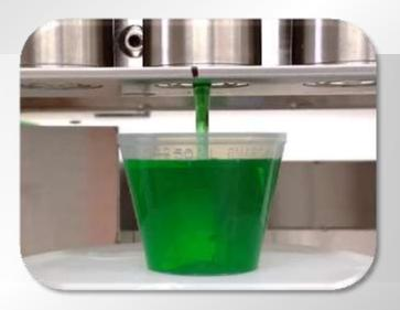
HMJ tech's 200 series AND 300 series valves have been purpose built to deliver the absolute best performance for dispensing. The unique internal design ensures laminar flow and clean transitions for perfect dispenses without drips or splashes. The all-stainless steel internals are chemically passivated for maximum performance with a wide range of fluids.
